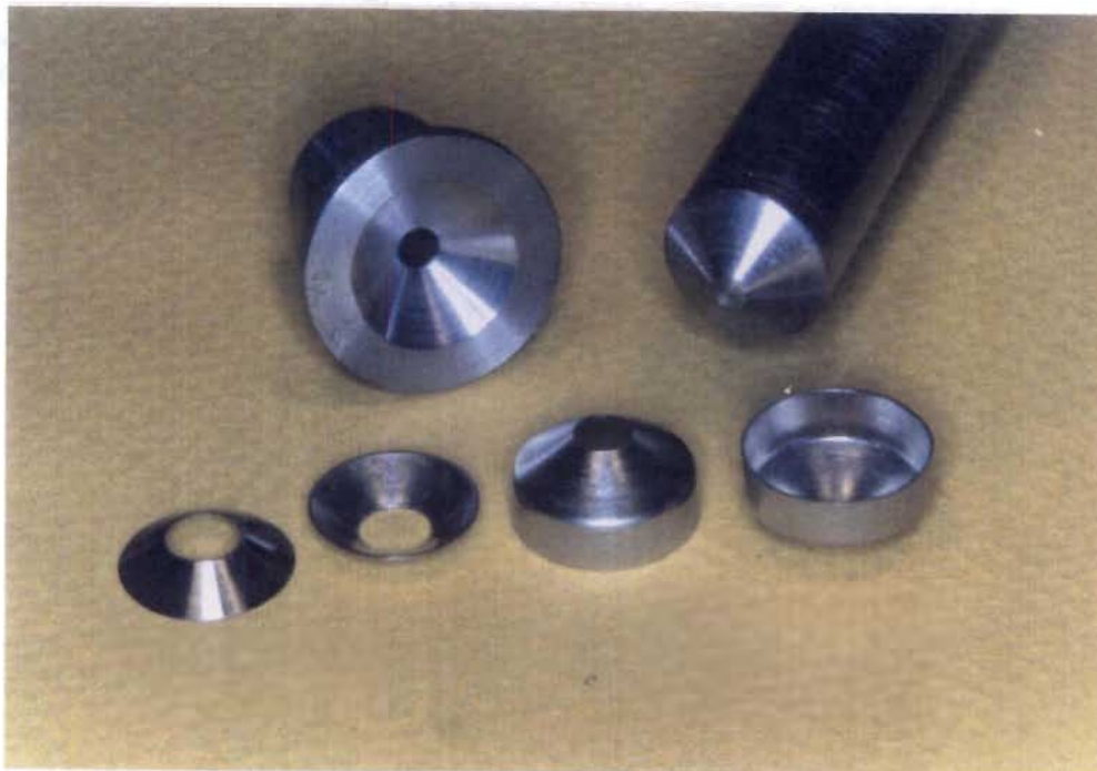
Figure 4.1 Focus Electrode, Switching Electrode and Final Die
