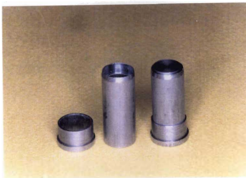
Figure 4.3 Cathode Holder Components and Assembly
