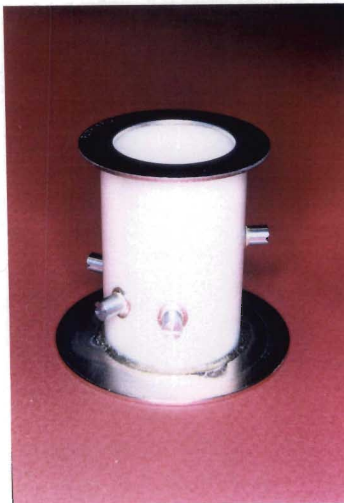
Figure 4.8 A Completed Vacuum Envelope with Connects
