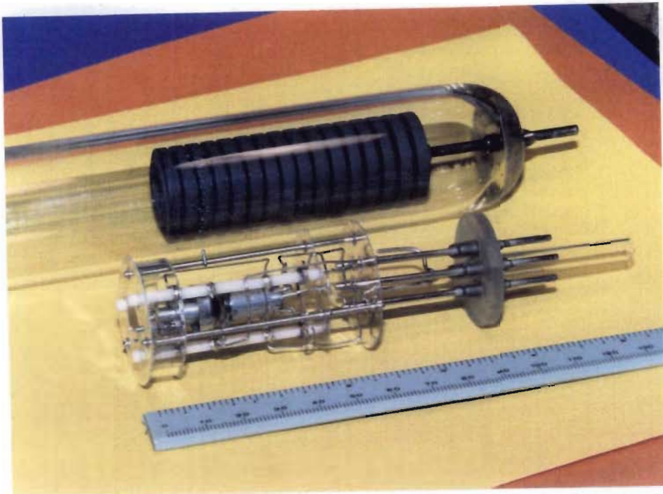
Figure 4.9 Completed Gun Module, Collector and Glass Envelope
