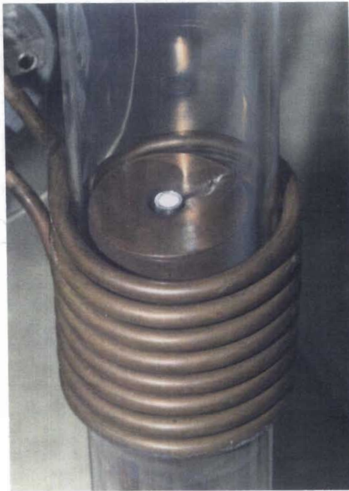
Figure 5.12 Aluminate Mix Inside Molybdenum Crucible in Induction Heater
