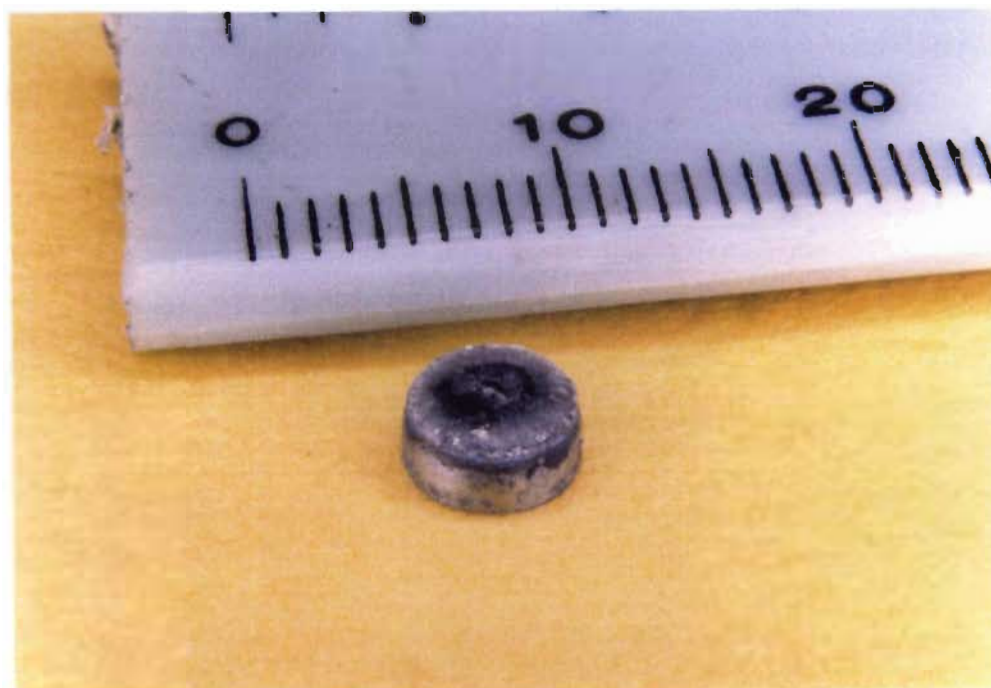
Figure 5.13 Cathode Pellet with Excess Impregnant on Top
