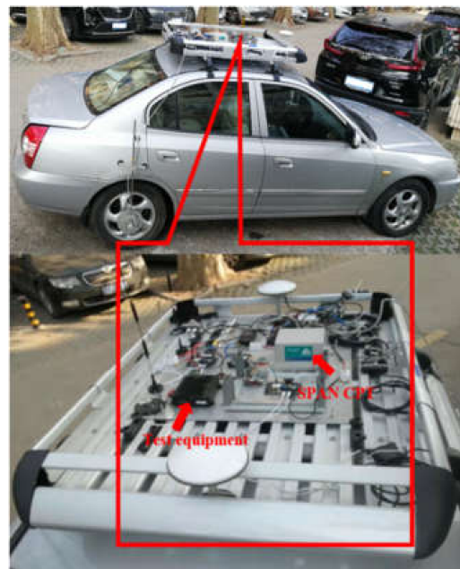
Figure 3. Data acquisition experimental platform.
