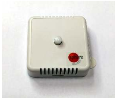
Figure 5: SPHERE Environmental Sensor node.
