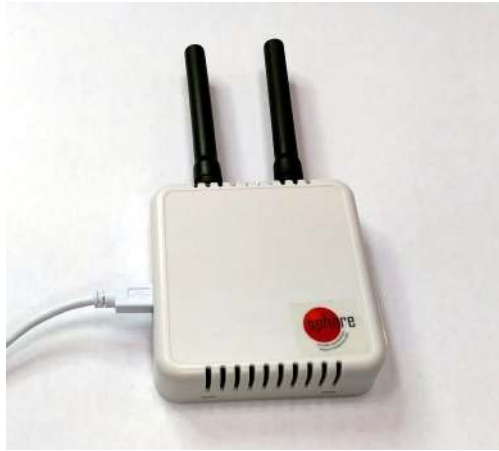
Figure 7: SPHERE Forwarding Gateway node.
