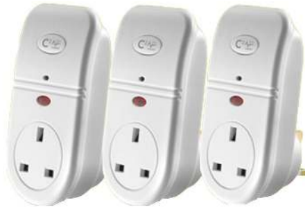
Figure 8: Appliance monitor ( CurrentCost ) sensor nodes.
