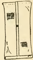
Fig. 5. Wire Cage made from a square of wire cloth by first folding edges together (as at a) to form a cylinder, and then cross folding the ends. It opens easily and closes securely with the fingers. Top edges should be woven or else there will be pricked fingers.
