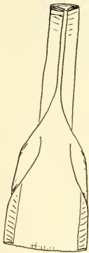
Fig. 3. A lifter, made by folding the edges of a rectangular strip of wire cloth, say 3 x 6 inches. The lower edge should be a woven edge. A tinner's shears and 4-inch folding tongs are the tools needed for making this and the two next following pieces of apparatus.
