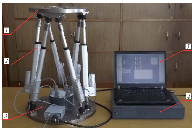
Fig.6. Stand equipment. 1 – operating platform; 2 – actuators; 3 – immobile base; 4 – connection and control interface; 5 – computer.
