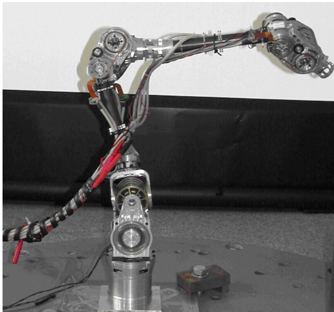
Fig. 7. Medical robot with external electronics (without housing).
