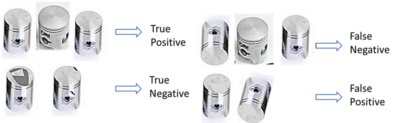
Figure 3. True positive, false negative, true negative, and false positive samples of the AC pistons.
