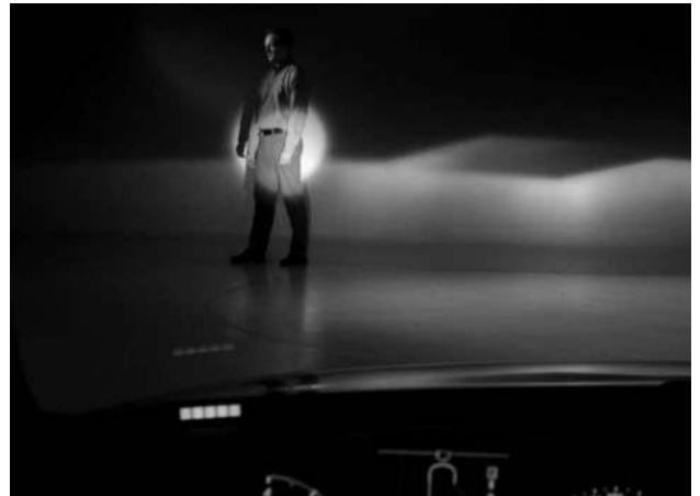
Fig. 2. Example picture of Volkswagen's "Marking Light"[3]
