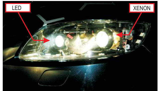
Fig. 3. Integrated prototype head lamp system
