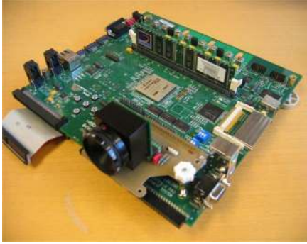
Fig. 11. Segmentation hardware is prototyped on an Xilinx VirtexII vp30 FPGA development board. A DDR memory is used for storing one frame of Gaussian parameters. A KODAK KAC-9648 CMOS sensor [39] is used to capture color image stream into the FPGA platform.
