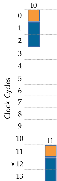
Figure 39 – Matrix-vector pipeline with II of 11, based on Intel (2016a).
