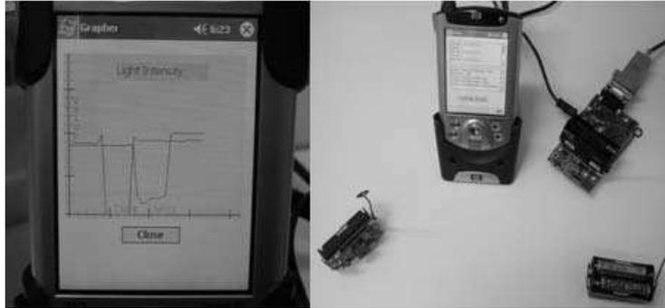
Figure 6.11 Mobile MoteCare Featuring a PDA Mobile Monitor
