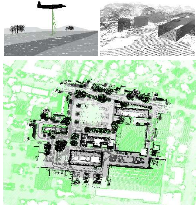
Fig. 9. Top left: Schema of the airborne based acquisition of reference data. Top right: 3D map consisting of aerial laser data and extrapolated 2D reference data. Bottom: Airborne and 3D map (green) with superimposed 3D scans (black).
