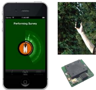
Figure 8: Prototype app interface showing the real-time feedback presented to the user during a 60 second survey, indicating the detection of a cicada song, and the electronic cicada that replicates the sound of the cicada, used for user testing.
