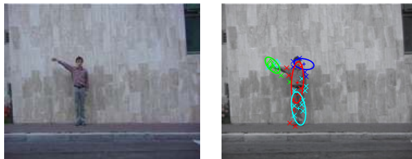
Figure 1. Recognizing human action classes: A sample frame and a four part model for hand waving over imposed on the original image. Static and dynamic features are shown, colored according to their part membership.
