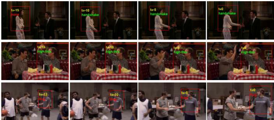
Fig. 7. Future action prediction visualizations. We show predictions of our method at different temporal stages before the action is executed (in yellow). For example, t = -15 in the first image denotes that the image is taken 15 frames before the action (handshake) starts. Correct predictions are shown in green and incorrect predictions in red. The last row shows examples of failure.
