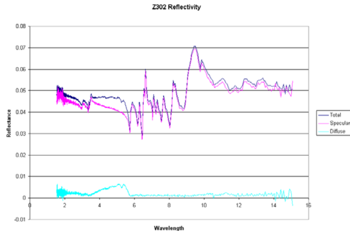
Figure 6: Z302 total, specular and diffuse reflectance at 8° incidence angle from 1.7 to 15 μm.
