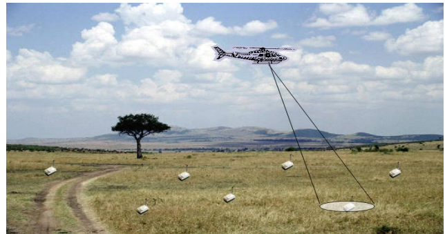
Figure 1. Localization of a sensor network using the Spotlight system
