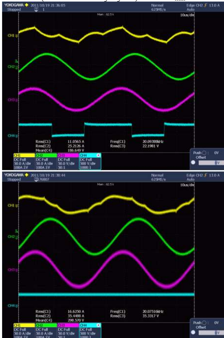
Figure 15. (Top) P=2\text{kW} , (Bottom) P=5\text{kW} @ v=246\text{mm} h=0\text{mm} . Top to bottom trace, I_b (Figure 4), I_1 (Figure 4), I_2 (Figure 5), and V_s (Figure 5) (inverse of duty cycle). k=1.14k_{\min} .
