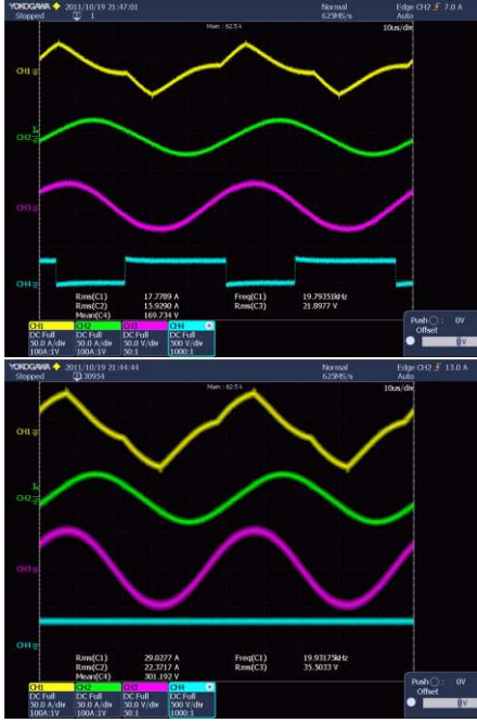
Figure 14. (Top) P=2\text{kW} , (Bottom) P=5\text{kW} @ v=172\text{mm} h=0\text{mm} . Top to bottom trace, I_b (Figure 4), I_1 (Figure 4), I_2 (Figure 5), and V_s (Figure 5) (inverse of duty cycle). k=2.0k_{\min} .
