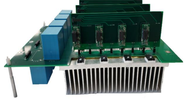
Fig. 12. Experimental prototype picture of a 20-kW hybrid Si/SiC switch based ANPC inverter.
