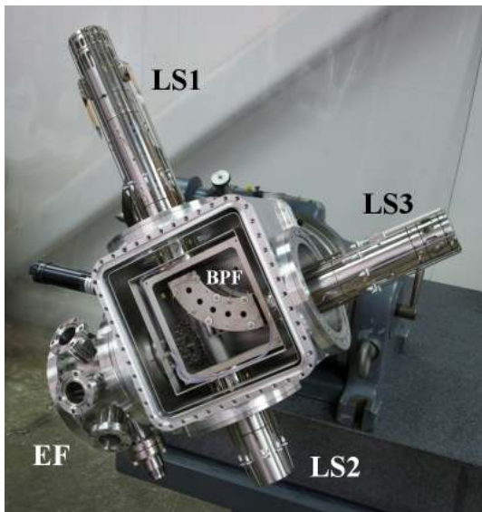
FIG. 6: (color online) Photograph of the TOF lens system. Magnetic shielding and vacuum enclosures removed for view. EF: electrical feedthru ports.
