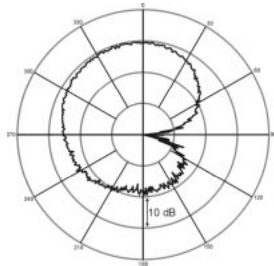
Fig. 6. Radiation pattern of an antenna on a high-impedance electromagnetic surface. The frequency is 2.44 GHz.
