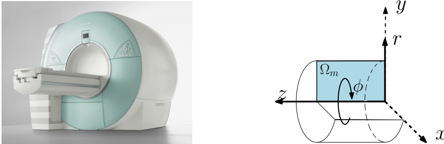
Figure 4.2: Transformation from a full 3D MRI scanner to the 2D axisymmetric case. Under simplifications of geometry, and neglect of certain excitation currents, the problem is constant in the azimuthal \phi -direction and can thus be axisymmetrically projected onto the meridian domain \Omega^m .
