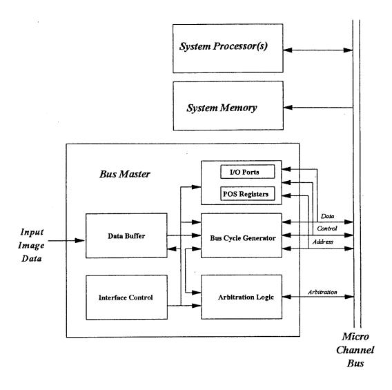
Figure 1. Micro Channel bus master system diagram
