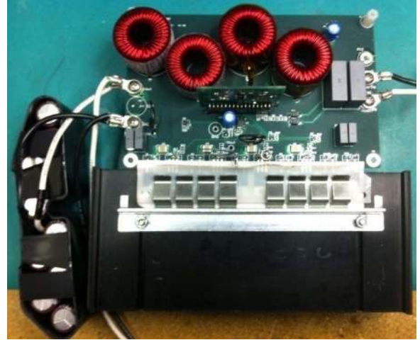
Fig. 12. Breadboard prototype of the BLIL PFC boost converter.
