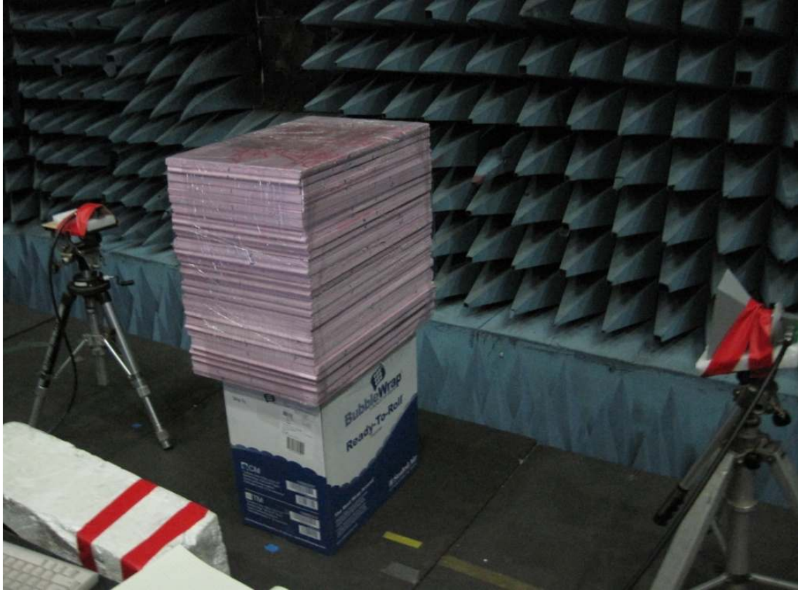
Figure 12. Test setup showing fully assembled lens, transmit and receive horn antennas
