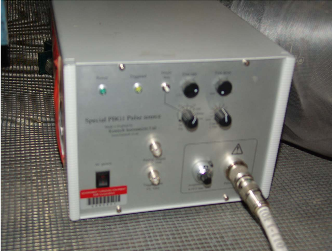
Figure 78. Special PBG1 Pulse Source Used in Impulse Tests
