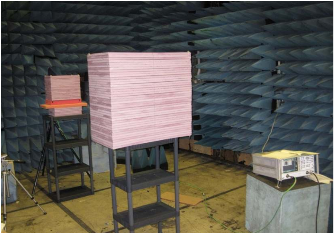
Figure 60. Test Setup; Lenses Positioned for Beam Collimation
