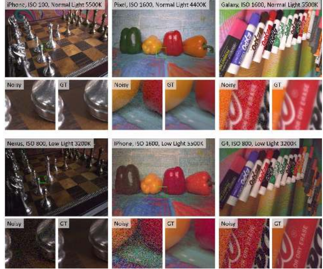
Figure 2: Examples of noisy images from our SIDDD dataset captured under different lighting conditions and camera settings. Below each scene, zoomed-in regions from both the noisy image and our estimated ground truth (Section 4) are provided.
