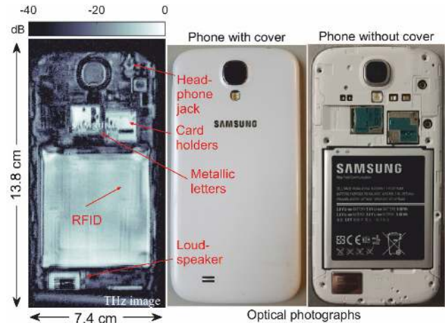
Fig. 9. Left: THz reflection image of a cell phone at 504 GHz. The image was recorded through the back cover of the phone, with the phone as shown in the photograph in the middle. The photograph on the right shows the interior of the phone with the back cover removed. Features such as the loudspeaker, the metal holders for SIM and memory card, various semiconductor chips as well as the headphone jack (invisible in the optical image) can be identified in the THz image. Furthermore, an optically invisible RFID loop antenna can be seen to be embedded under the cover of the phone’s battery. The overall dynamic range of the image exceeds 40 dB.
