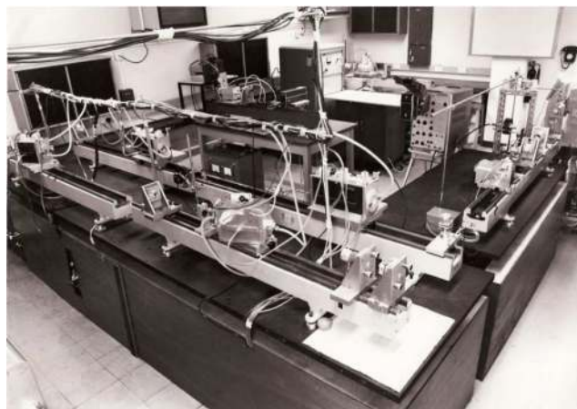
Figure 5. An early ~100 mJ, 5 ps flashlamp-pumped Nd silicate glass laser built by Roy Taylor at Imperial to investigate high harmonic generation (HHG; 2nd, 4th, 28th in Ne or He). (Picture courtesy of Imperial College London.)
