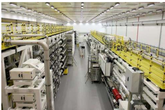
Figure 42. The Orion Laser Hall showing the long pulse beamlines on the left and the two petawatt beamlines on the right. (Picture courtesy of AWE.)
