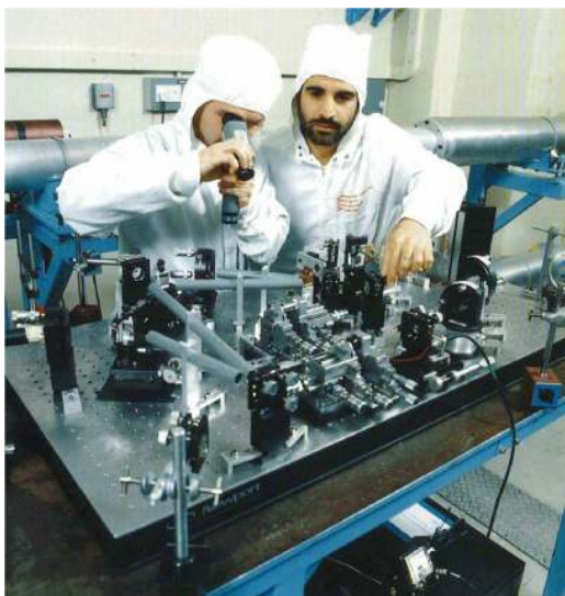
Figure 13. Dave Hughes, Research Fellow, and PhD student A. A. Majdabadi from Southampton commissioning the Nd:LMA oscillator on the VULCAN laser for ultra-short pulse operation. (Picture courtesy of STFC.)
