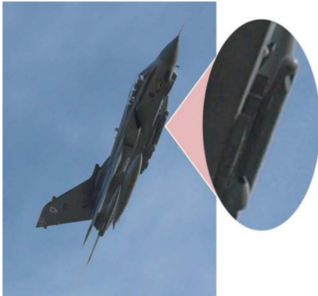
Figure 79. TIALD mounted on a Tornado. (Picture courtesy of Leonardo.)
