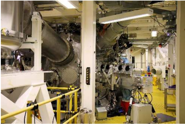
Figure 43. The Orion 4 m diameter target chamber. (Picture courtesy of AWE.)
