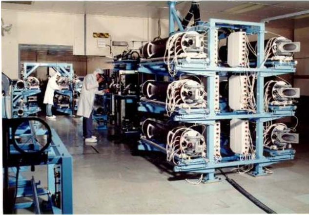
Figure 31. The VULCAN laser hall showing the output disc amplifiers with Colin Danson, foreground, and Bob Bann carrying out final system alignment circa 1986. (Picture courtesy of STFC.)
