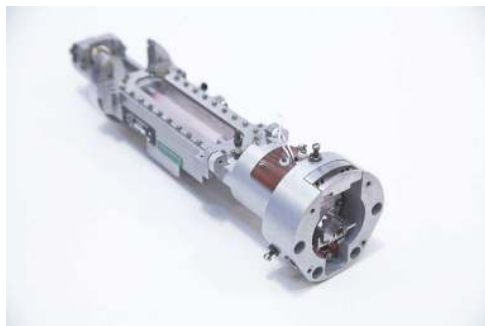
Figure 73. The Ferranti version of the Westinghouse Nd:YAG laser acquired via a radar for laser swap in 1966. The Porro is visible on the right-hand side while the mirror is at the far end. The Nd:YAG rod and pump chamber are visible in the centre of the structure. (Picture courtesy of Leonardo.)
