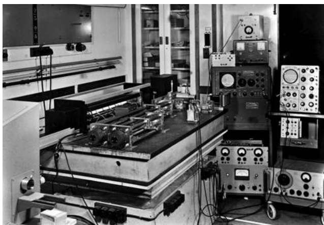
Figure 1. Ed Ballik's 1.15 \mu\text{m} HeNe laser at Oxford 1963–1964. (Picture courtesy of the University of Oxford.)
