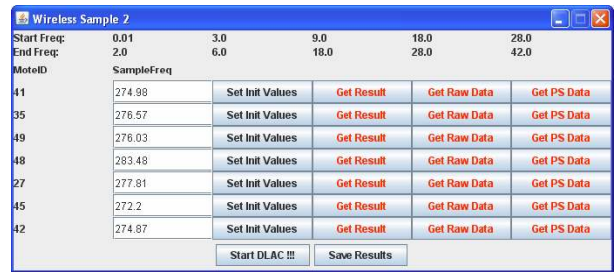
Fig. 6. The damage localization user interface
