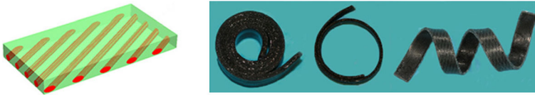
Fig. 1 Design and experimentally observed cylindrical, equilibrium shapes of 3d-printed composite bilayer plates. Reproduced from Ge et al. (2013), with the permission of AIP Publishing
