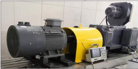
Fig. 15. Test rig: M22 SynRel motor (left hand side) and 160kW induction machine used as a load (right hand side).
