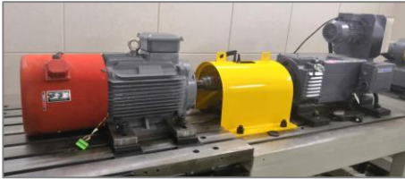
Fig. 14. Test rig: M21 SynRel motor (left hand side) and 40kW induction machine used as a load (right hand side).
