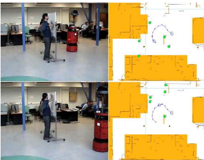
Fig. 17. Robot is invisible to the human. To avoid any unpleasantness coming from the sudden appearance of the robot, the planner calculates a path which make the robot appear farther.
