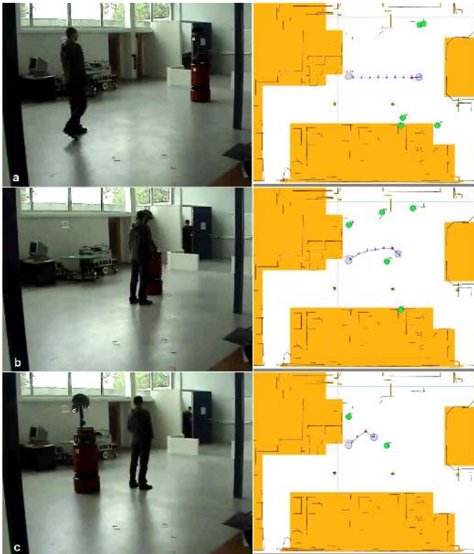
Fig. 16. A person and robot move toward each other. The robot changes its trajectory to avoid a collision. After passing next to the human instead of taking immediately its previous lane, it gives a little distance to the human. This behavior ensures a comfortable and riskless motion for the human.
