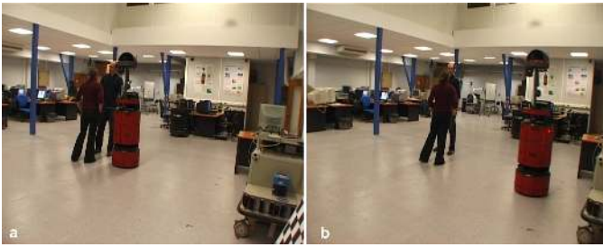
Fig. 13. A comparison between a classic motion planner and the Human Aware Motion Planner which produces a more acceptable path by taking into account the safety and visibility of each human in the environment.
