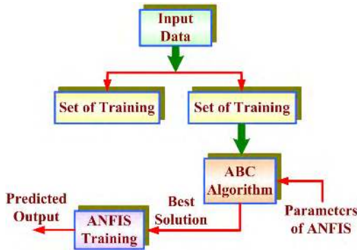
FIGURE 6. Complete structure of Hybrid ANFIS-ABC control.
