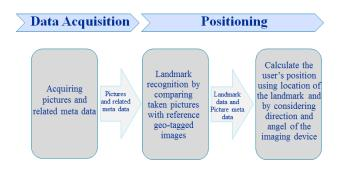
Figure 1. Traditional approach of visual positioning.
