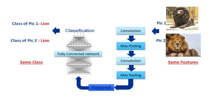
Figure 2. Same features lead to recognize a same class by a pure Neural Network approach.
