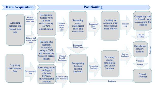
Figure 4. Proposed conceptual framework for visual positioning using ontology
