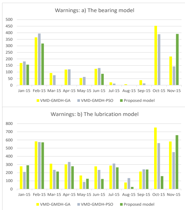
FIGURE 13. Comparison of a) the gearbox bearing model and b) the gearbox lubrication model in terms of warnings.
