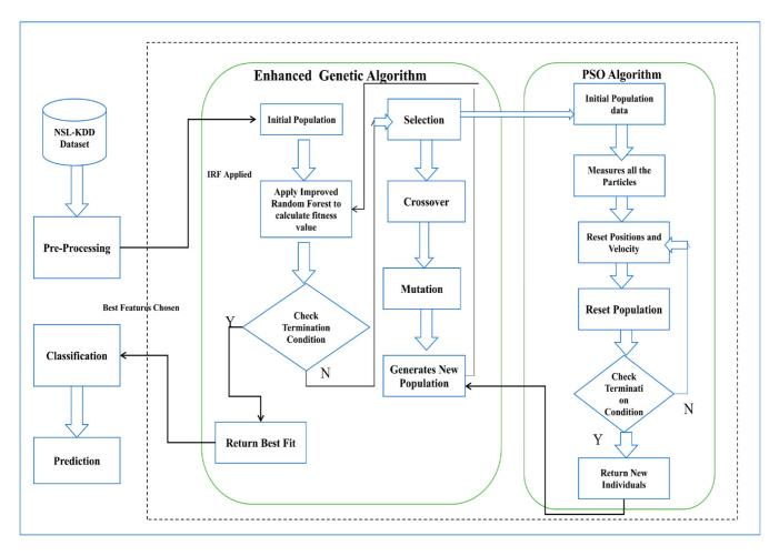
Figure 2. The working of the proposed hybrid IDS model.
