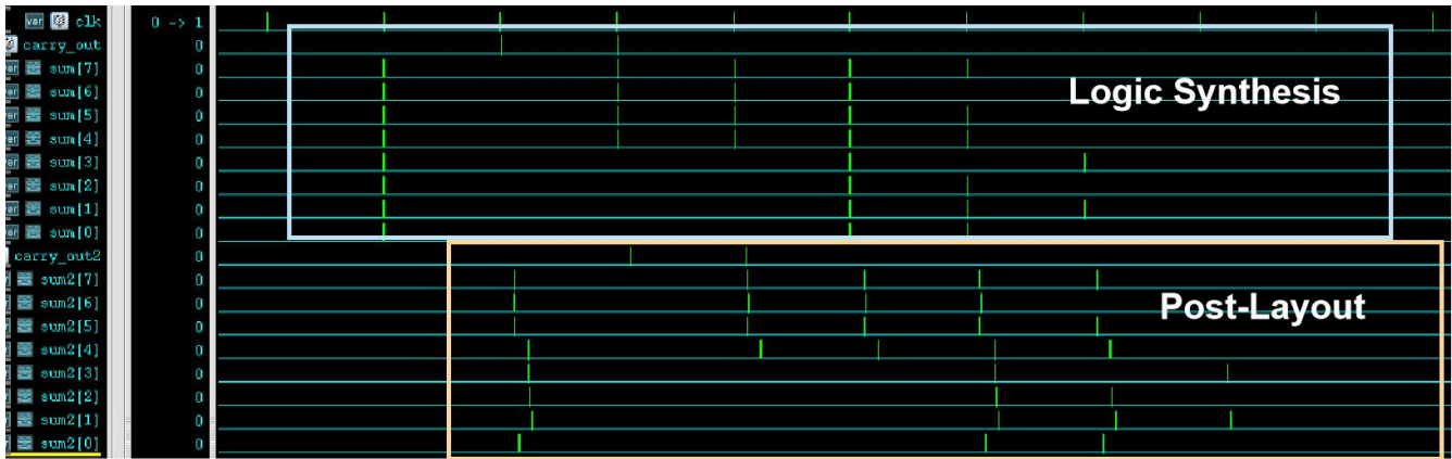
Fig.19. Waveform comparison between logic synthesis netlist and post-layout netlist (8bit-ALU).
