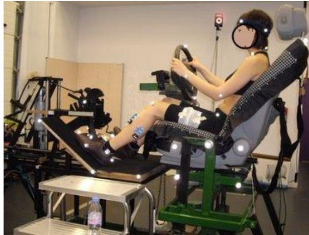
Figure 4.1: Overview of the adjustable vehicle mock-up (reproduced from the DHErgo Newsletter n.2).
