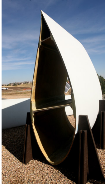
Figure 4.1: Photo of an actual wind-turbine blade cross-section taken at NREL in Golden, CO, USA. Credit: Green Career Central ( http://www.greencareercentral.com ).
