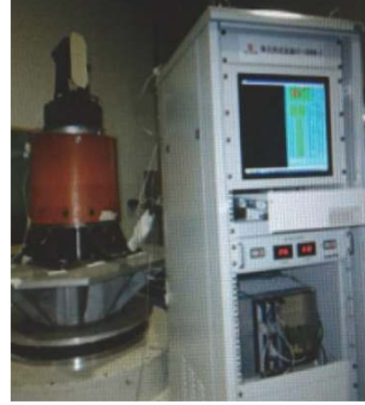
FIGURE 1: The employed instrument containing servo turntable for missile-borne radar.
