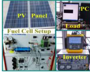
Fig. 9. Lyapunov-based single-stage PV-fuel system.
