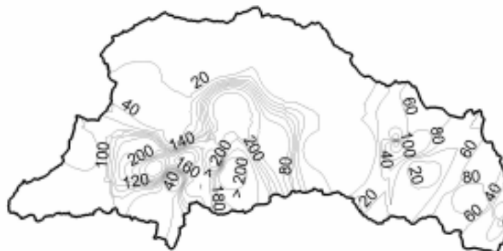
Figure 8 Estimated return periods for maximum daily peak discharge during February 2000 in the Sabie River catchment
