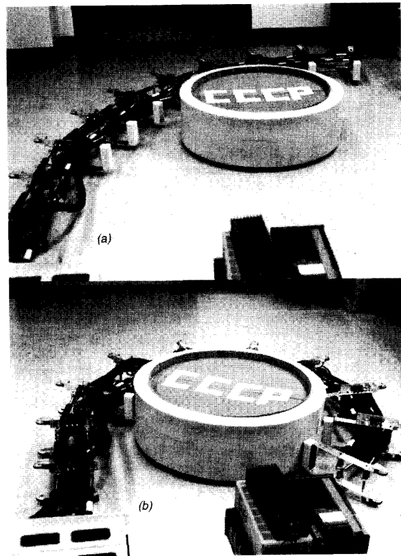
Figure 5. Single-arm grasping/manipulation, e.g., satellite recovery.
