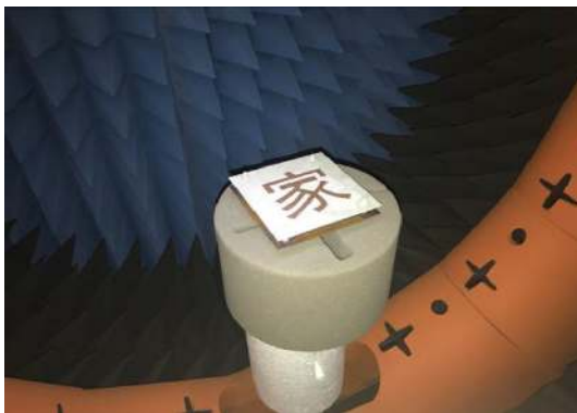
Fig. 14. Photograph of a fabricated dual-band Jia-shaped patch antenna under measurement.
