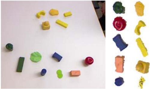
Figure 1. An example of an RGB-D object identification scene. Columns on the right show example segments, identified as positive (far right) and negative (center).
