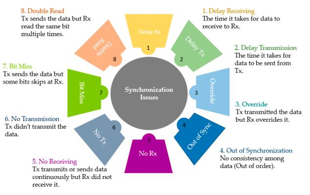
Figure 2. Detail of the synchronization errors during interprocessor communication.
