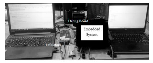
Figure 6. Emulator environment where two emulators connected with two PEs.
