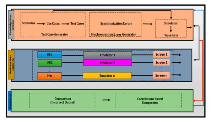
Figure 4. Steps for detection and localization of the errors.
