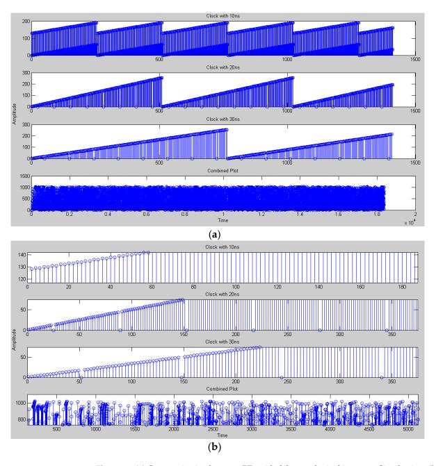
**Figure 12.** (a) Communication between PEs with delays and miss bit errors—Simple view. (b) Communication between PEs with delays and miss bit errors—Expanded view.
