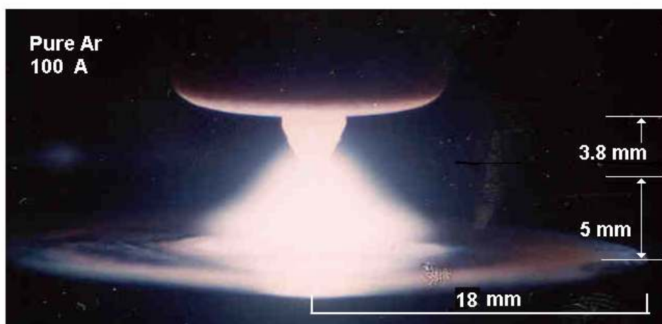
Figure 7.1 A 100 A argon TIG arc, with typical dimensions
