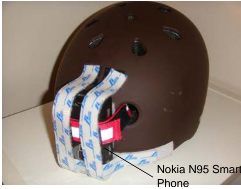
Figure 1: Sensor helmet for collecting activity data.
