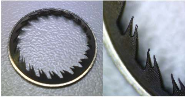
Fig. 7 Prototyped steel teeth ring, using tooth geometry J (Fig. 10, bottom), 2.0 mm height, 1.4 mm width, 0.3 mm spacing between teeth, and 45 deg inward angle. The ring has 21 teeth.
