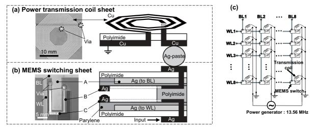
**Fig. 3: The power transmission sheet comprising (a) power transmission coil sheet and (b) MEMS switching sheet.** Pictures and crosssectional illustrations are shown. A: Electrodes for electrostatic attraction connected to the word-line (WL) and bit-line (BL) of MEMS switch. B and C: Electrodes for power transmission connected to coils and a power generator. (c) The circuit diagram of the power transmission sheet. A frequency of 13.56 MHz is used in the power transmission system.
