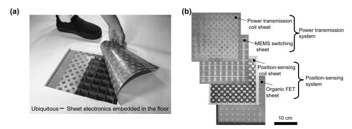
**Fig. 1:** *Wireless power transmission sheet*. (a) An image of the world's first large-area *wireless power transmission sheet* embedded in the floor. A part of the cover layer is peeling off. (b) A picture of the device assembly comprising a power transmission system driven by an  $8 \times 8$  MEMS-switching matrix and a position-sensing system driven by an  $8 \times 8$  organic FET active matrix. The power transmission area is  $21 \times 21$  cm<sup>2</sup>.
